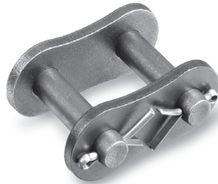
CCL Connecting link with cotter. Slip-fit
